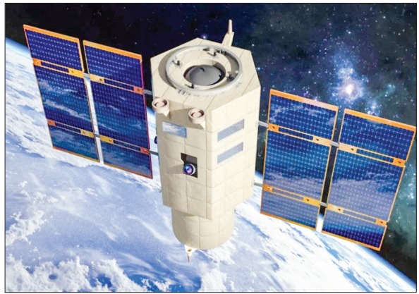
Elbit’s JUPITER space camera launched from Vandenberg, California, SpaceX. cameras. It features an exceptionally large optical aperture, lightweight design, and seamless integration with satellite systems and ground stations. According to Elbit, the data produced by JUPITER is optimized for advanced image-
